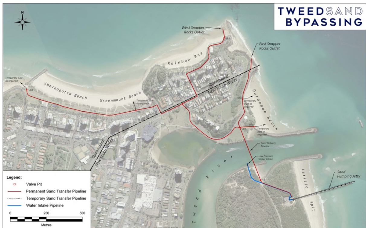
Figure 1.1 Fixed sand bypassing system (TSB, 2024)
