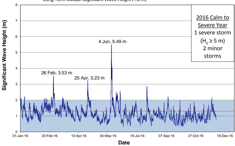
Note: The significant wave height is defined as the average height of the highest one-third of waves recorded over a period of typically
