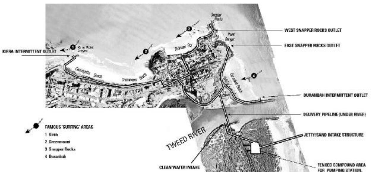
Figure 2 – Layout of Sand Bypassing System
