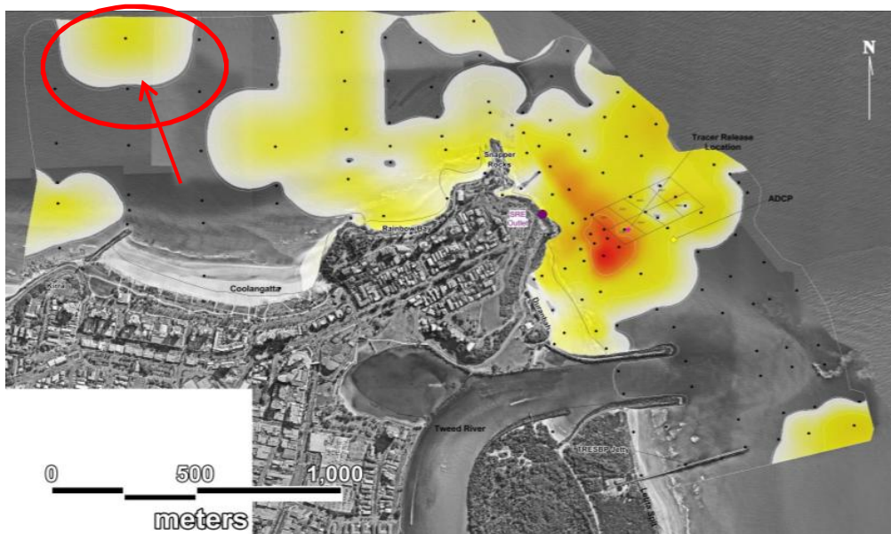
Figure 3-14 Tracer material concentrations 9 months after release (HaskoningDHV, 2017)
