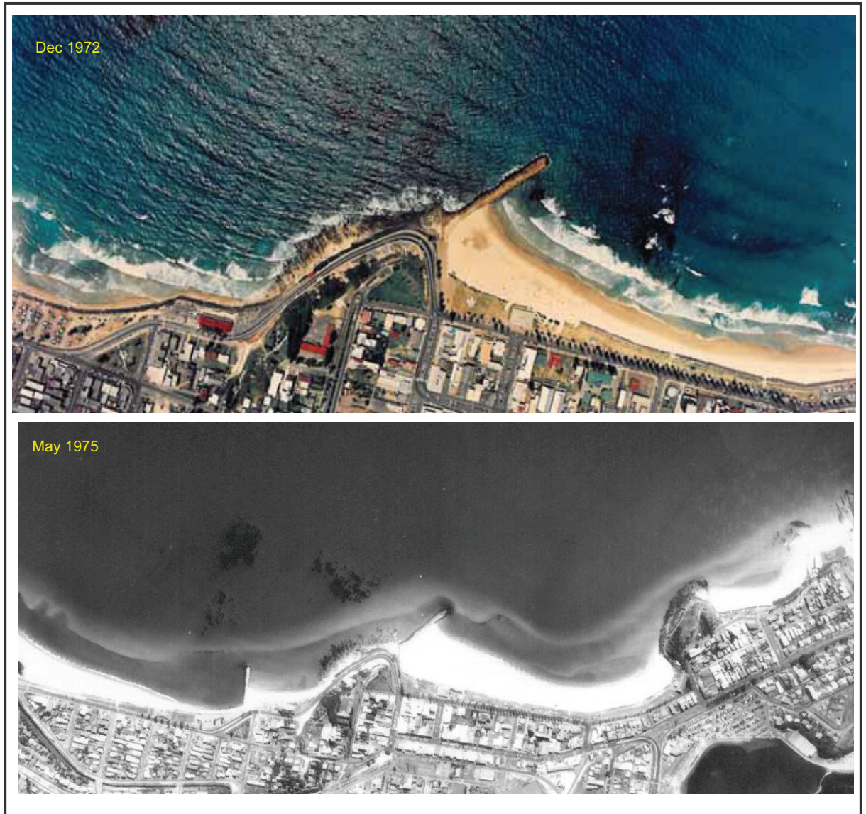
Figure 7 Sand movements post Kirra Groyne construction 1972 - 1975
