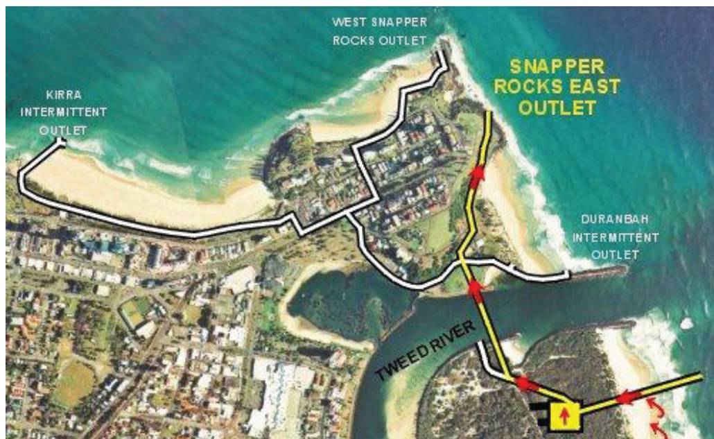
TRESBP pipe network with the main sand bypassing route shown in yellow.
