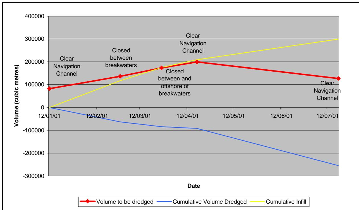
Figure 3: Plot of cumulative dredging volumes, cumulative infill volumes and volume to be dredged over the period 12/1/01 – 19/7/01.
