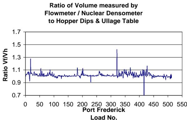
**Figure 3 : Ullage Flowmeter Comparison**
