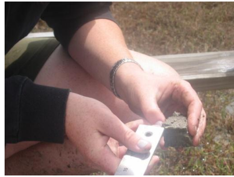
Figure 7: Mini-core removal and measurement.
